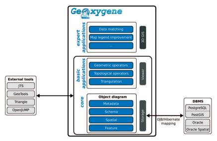
Figure 3.7. GEOXYGENE platform's general structure
