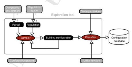
Fig. 1 Global schema of our proposition to produce a database of building configuration according to a regulation exploration space
