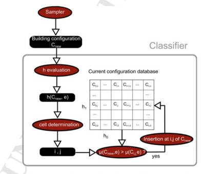
Fig. 4 Classification steps applied on a configuration with a 2 dimension variety function
